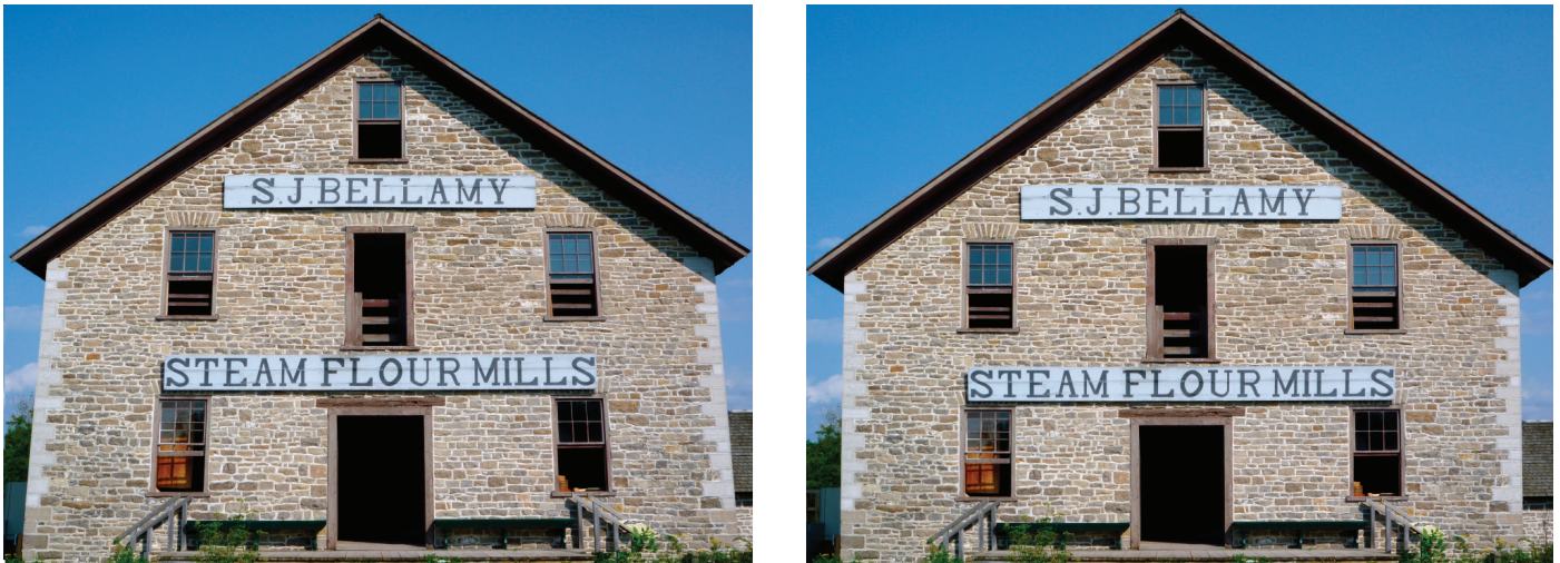
Figure 18 Original image with vertical camera tilt (left) and after distortion correction (right)
